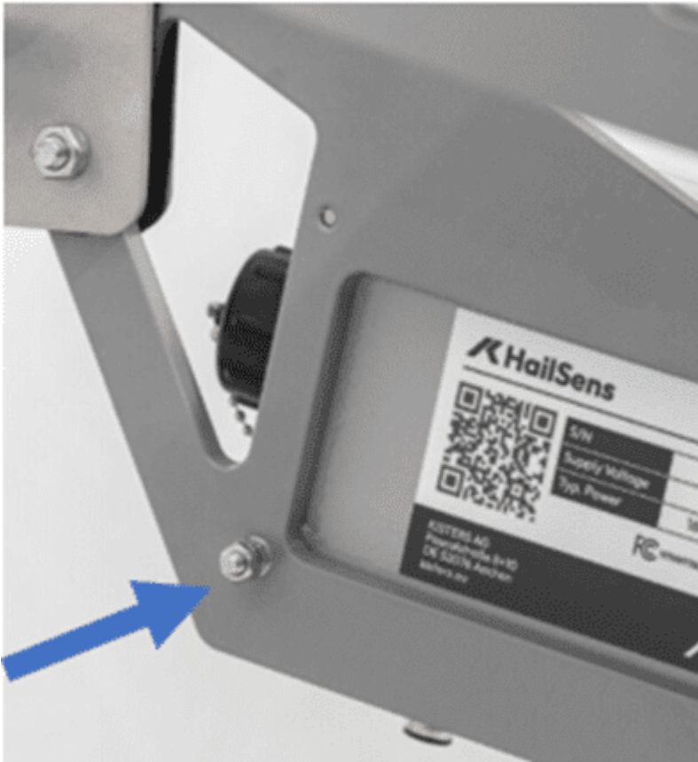
Figure 4 – Earthstud on rear-side of electronics box
