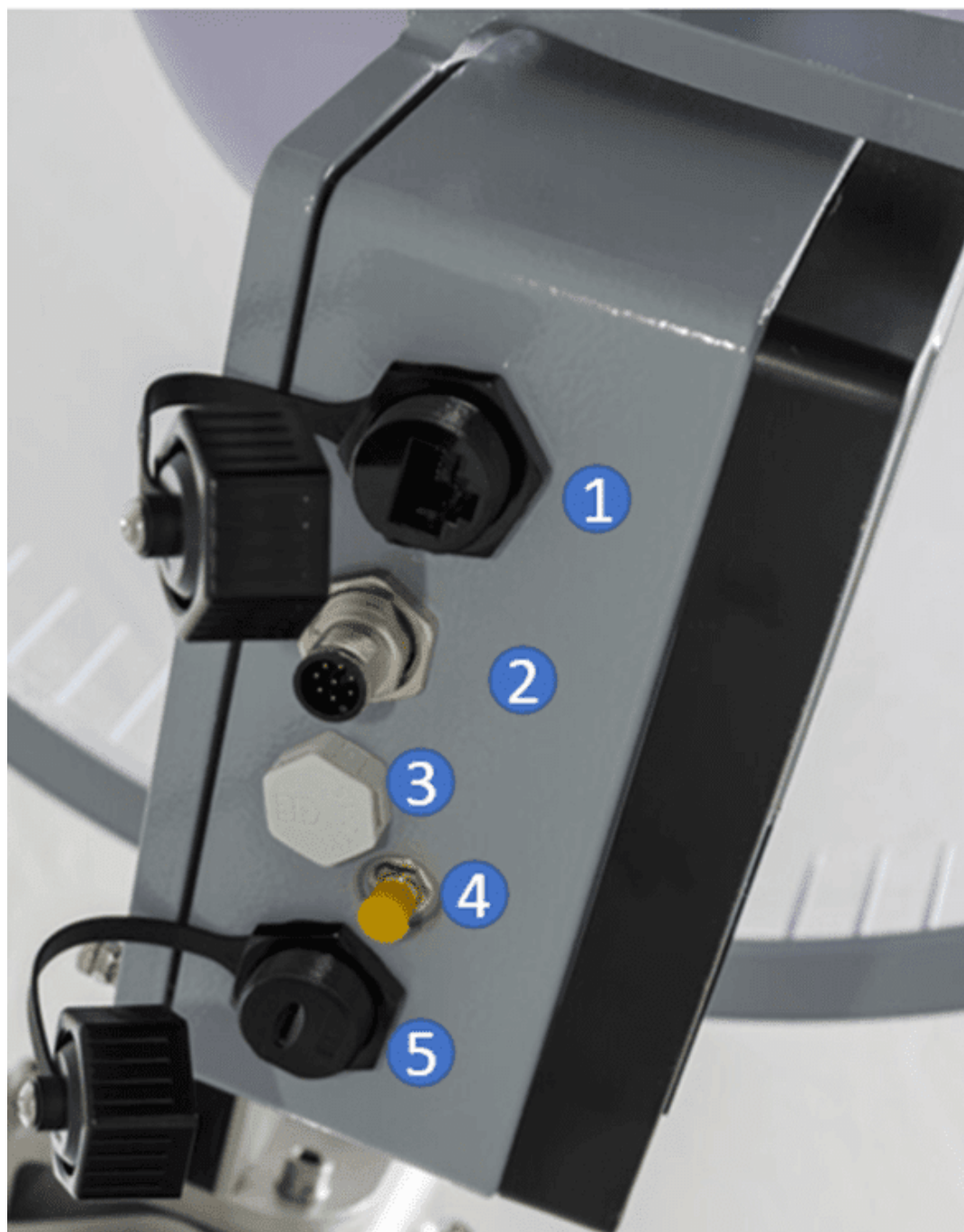
Figure 3 – Bottom side of electronics board with input/output connectors
