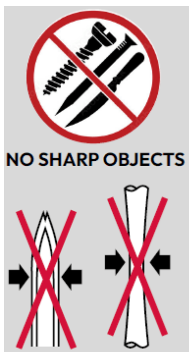
Figure 4 – Installation: No sharp Objects. Do not pinch the cable.
