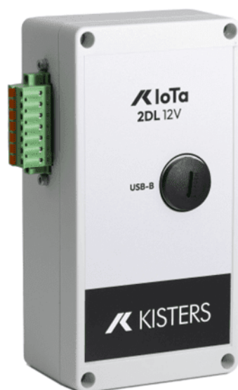
Figure 1 – IoTa 2DL 12V SensorNode in portrait view with labelled connectors at the left side
