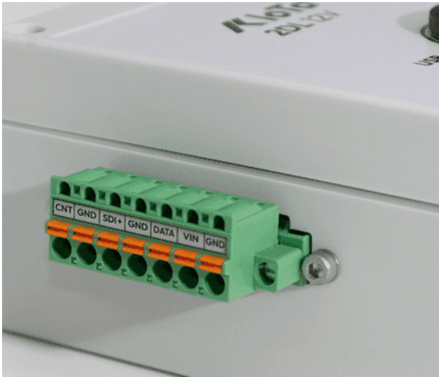
Figure 2 – labelled 7-pin terminal of the IoTa 2DL 12V SensorNode's left side
